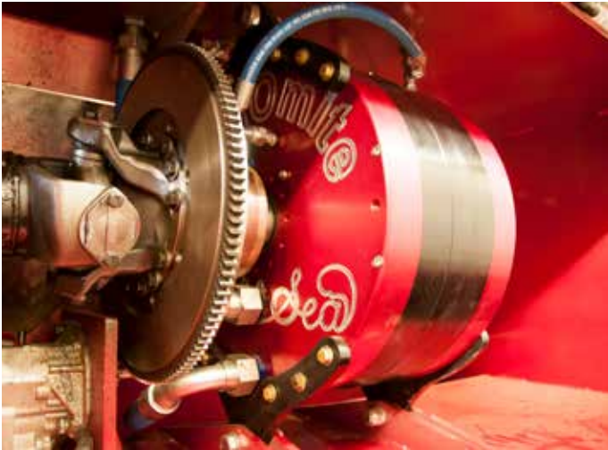
The core of the power bench consists of a water brake specially developed for the sport.
